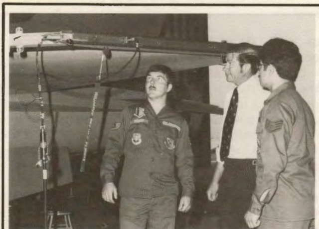
Functional check-out being performed on F-16 wing tip launcher.
