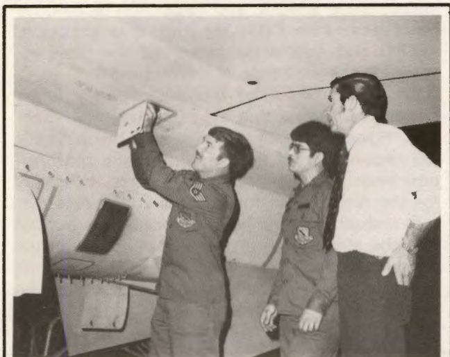
SSgt D. J. Romero and General Dynamics Crew Chief, Mr. P. Vercher, look on while SSgt T. H. Duggin installs refuel receptacle cap.
